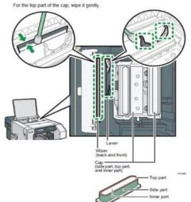
For Regular Maintenance, use the cleaning tool, two cleaning pads, and cleaning liquid. Discard the cleaning pads when done – do not reuse them.
